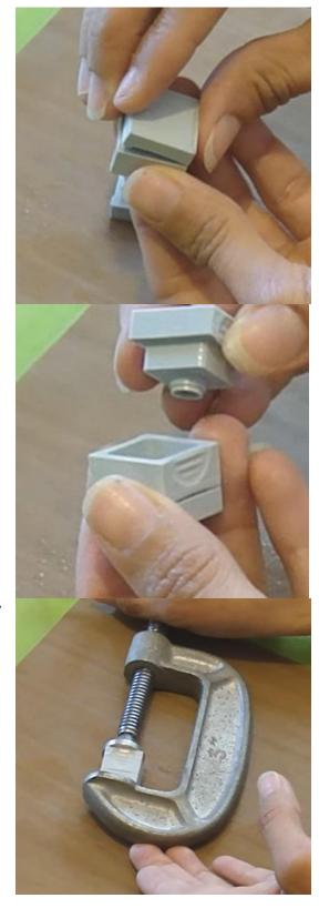
9. Now place entire mold upside down on table and slowly pull out bottom layer while holding the finger grip of the middle layer. The main thing here is to remove the bottom layer before the top layer so that clay becomes attached to the top layer.
