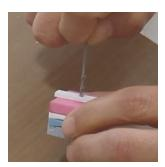
5. After it is dry reassemble box with drill bit guide and hand twist drill bit through box again. This is to compensate for any shrinkage that may have occurred during drying.
