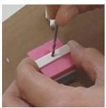
2. Using the provided drill bit, hand twist the drill bit through wet clay till it comes out other side. Literally remove the drill bit from the other side you started from passes through the box.
