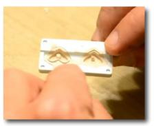
13. Separate the layers carefully and dry on the hot plate for a few more minutes
