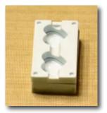
2. Carefully lubricate all three parts of 3. Place a quantity of clay the hollow heart builder mold using Cool Slip or olive oil. Then clip the top layer to the middle layer.
