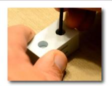
8. Replace the top layer; turn the mold up side down, and using a 3 mm or slightly bigger drill bit press the extruded clay back in. Remove the excess.
