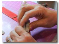
12. Open the top layer, remove the excess clay and set on the hot plate to dry for approximately 10 minutes
