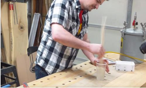
**Mixing:** Combine part A and B together into a mixing cup and begin mixing. Continue mixing until all striations disappear and resin is clear. Scrap sides, bottom, and excess resin off stir stick often to ensure that all resin is mixed. **Note:** Mixing, pouring, and pressurization of pressure pot should be done within the stated working time of the resin.
