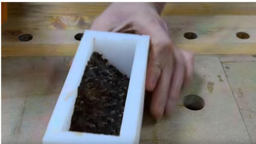
**Prepare Wood:** Before starting, dry and stabilize wood. Using available saw, trim wood to fit into mold-box. If using scraps, chips, or fines, simply pour them into your mold box. **Note:** Moisture in any substrate will cause bubbles in resin, therefore we recommend that humidity be less than 5% and/or stabilize wood.
