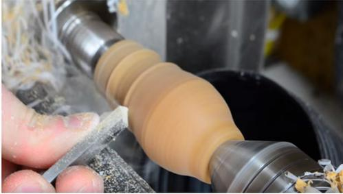
**Turning:** To ensure that the highest cured properties have been achieved, it's recommended to allow resin to cure for 12-24hrs. before turning.
