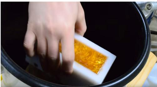
**Pressurize:** Place mold inside of pressure pot and pressurize to 40-60 psi. Many pressure pots have their air inlets in the lid, therefore introduce air slowly to avoid blowing resin out of your mold box. A deflector can also be placed over the mold box to divert air away from resin. Hold pressure until resin has hardened and can be demolded. Resin must cure under pressure to avoid visible air bubbles in your cured blank.
