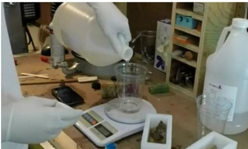
**Measure Resin:** Estimate (or use Volume Calculator on Alumilite.com) the amount of required resin to fill the mold-box and measure out side A and B per the instructions for the respective resin. Alumilite Clear is 1:1 mix ratio by weight, therefore you will need to weigh each side to achieve an accurate mix ratio. **Note:** improper mix ratio can result in tackiness, cloudiness, and soft resin.
