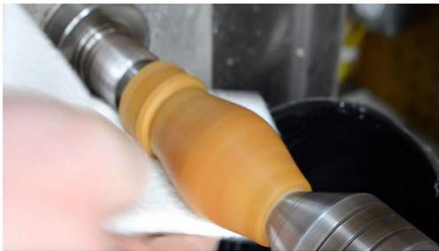
**Sanding & Polishing:** Alumilite resins can be sanded using fine grit sanding paper or pads. Plastic Polish such as Novus can be used to polish Alumilite Clear to a high gloss.
