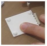
4. The notches at end of roller are spaced 4mm apart when measuring from center of notch. With these you can multiple hinge blanks. Also to expand hinges you would skip a notch to create 8mm blank. Place roller with notch side parallel to snake to make measured cuts
