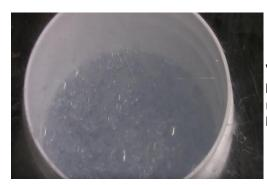
**Vacuum Degassing (if available):** Once Amazing Clear Cast has been thoroughly mixed, if you have vacuum degassing equipment, we recommend degassing prior to pouring to minimize air bubbles. If you do not have this equipment, proceed to next step.
